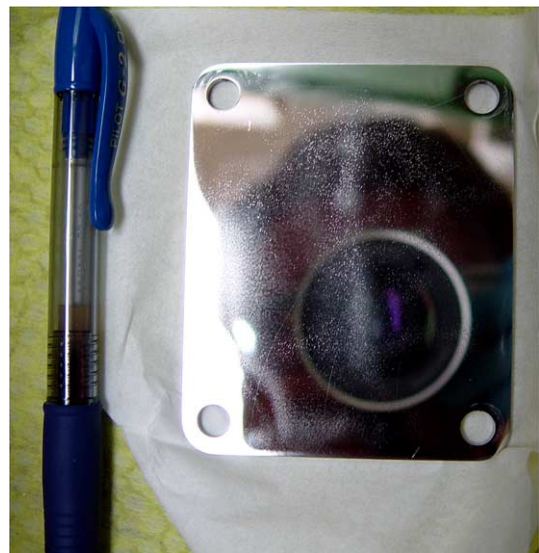
Fig. 5. Photograph showing severe pitting damage along the beam direction on the bottom surface of the 63-mm-wide × 76-mm-long × 3-mm-thick insert plate used in target TL from the June 2002 WNR tests.
